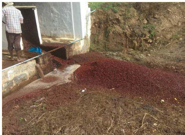
Fig. 2. Waste pulp is coming out of the unit after the pulping process.
